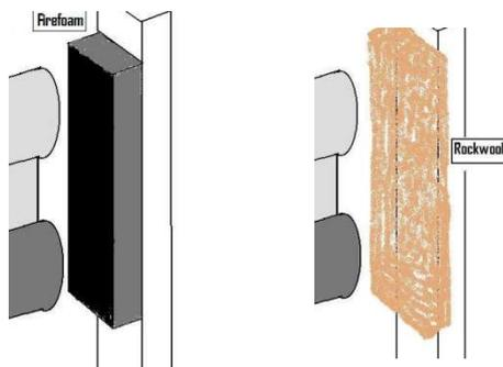
In the gap between the FB Cavity Vent and the stud, it should be used Rockwool or FireFoam. Between the under boards in board on board system you must use Rockwool or Firefoam to seal the gaps.
