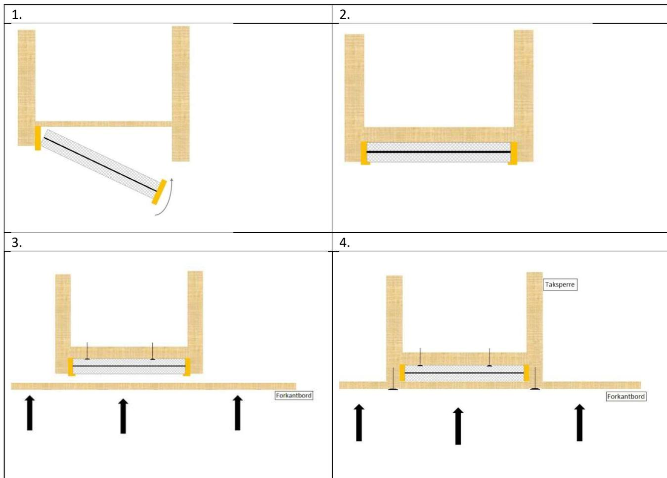
*The images below shows mounting behind vertical cladding.*
